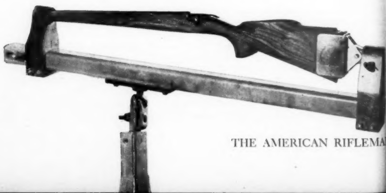
3 Adjustable cradle allows stock to be turned and moved into any position, permitting the worker to take advantage of convenient and comfortable working positions. A much simpler device is a 2x4, with suitable uprights for supporting the stock, which can be clamped in a vise
